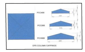
The above are ABPs' standard range of profiles. ABP can supply a limitless range of wall and column capping profiles provided an accurate template or design is supplied. These cappings are for single brick walls and if the requirement is for half brick or EPS walls this must be specified.
